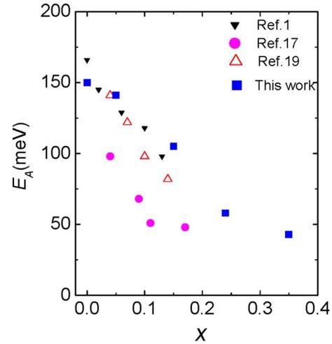
FIG. 3. (Color online) Energy level ( $E_A$ ) of Mg acceptors in Mg doped p- $\text{In}_x\text{Ga}_{1-x}\text{N}$  alloys as a function of In content  $x$ . Data from references available up to  $x=0.17$  are also included.
