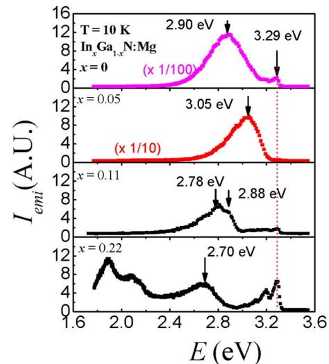
FIG. 4. (Color online) PL spectra of Mg-doped p-type  $\text{In}_x\text{Ga}_{1-x}\text{N}$  alloys measured at temperature 10 K.
