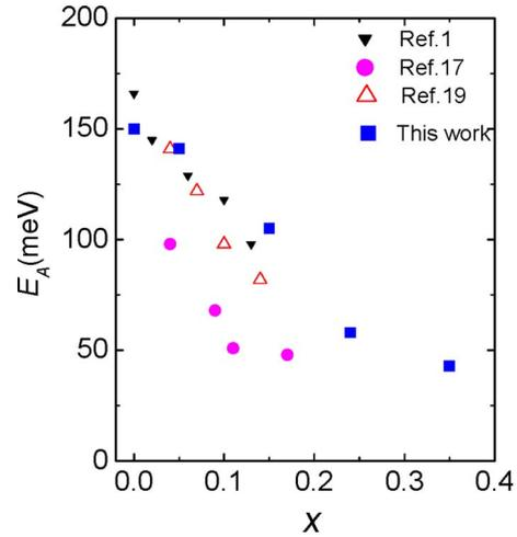
FIG. 3. (Color online) Energy level ( $E_A$ ) of Mg acceptors in Mg doped  $\text{p-In}_x\text{Ga}_{1-x}\text{N}$  alloys as a function of In content  $x$ . Data from references available up to  $x=0.17$  are also included.
