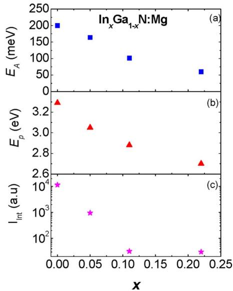
FIG. 5. (Color online) Mg acceptor energy levels  $E_A$ , peak position of Mg related emission  $E_p$ , and integrated PL intensity  $I_{int}$  as functions of In content  $x$ . (a)  $E_A$ , (b)  $E_p$ , and (c)  $I_{int}$ .
