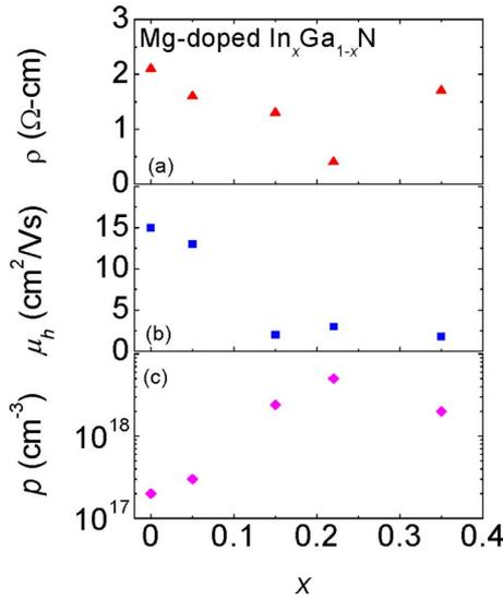
FIG. 1. (Color online) Room temperature (a) resistivity  $\rho$ , (b) hole mobility  $\mu_h$ , and (c) hole concentration  $p$  as functions of In content ( $x$ ) in Mg doped  $\text{In}_x\text{Ga}_{1-x}\text{N}$  alloys.
