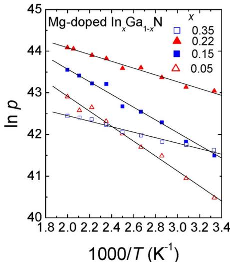
FIG. 2. (Color online) The Arrhenius plot of free hole concentration in Mg doped  $\text{In}_x\text{Ga}_{1-x}\text{N}$  alloys.
